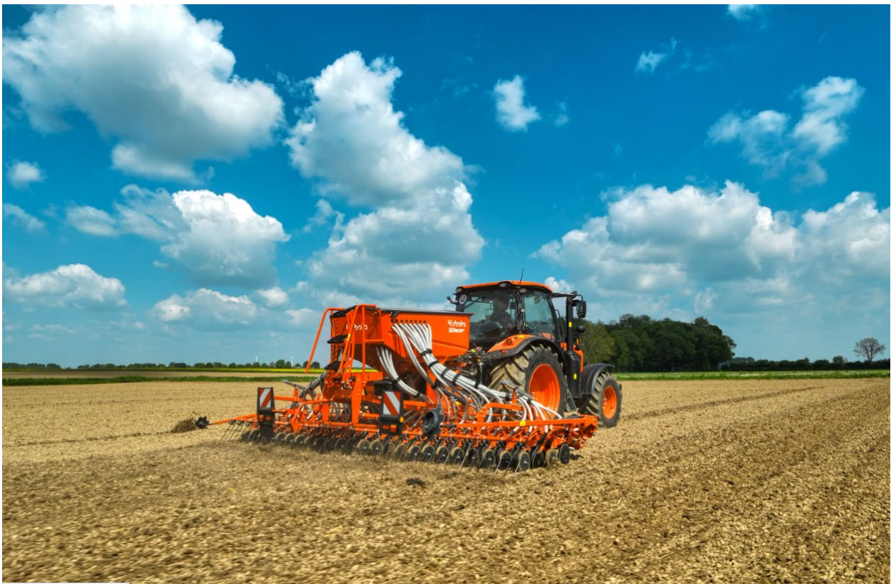
Image 1: Kubota SD1601F, 6.00m working width, e-com model, fully ISOBUS compatible
