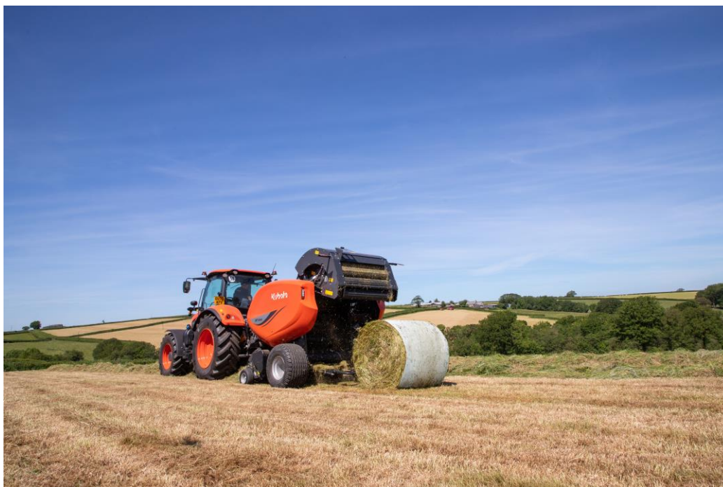
Picture: Kubota BF3500 producing high-density bales
