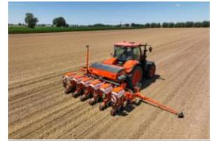
Image [Kubota-PP1451V-field](#) Kubota precision drill PP1451V with variable frame concept in field
