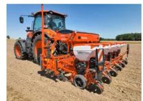
Image [Kubota-PP1451V-HD-II](#) Kubota precision drill PP1451V with HD-II row now with 60l hopper capacity
